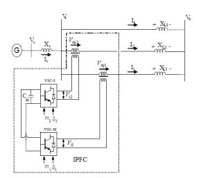
Fig.1 A single machine infinite-Bus power system installed with IPFC.
