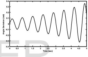
Fig. 5. Angle deviation without using PSS and IPFC
