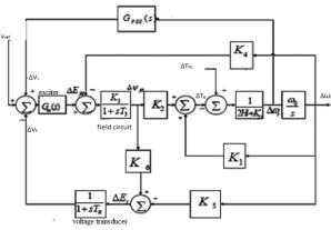
Fig. 3.control block diagram for power system stabilizer
